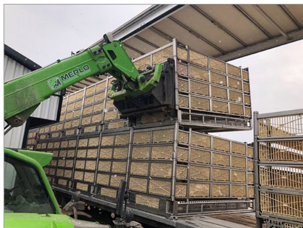
Figure 8. Placement of upper level Marel-Stork module on top of locator pins of first layer module to secure it for transport.
