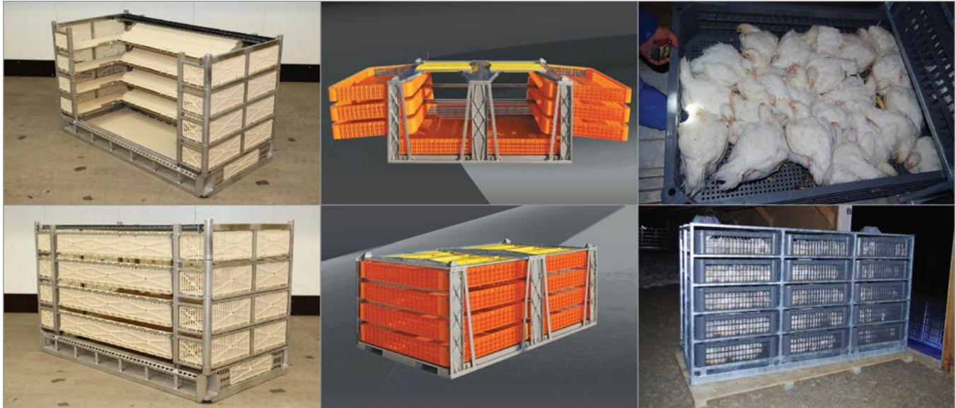
Figure 4. Example of Marel-Stork module, Meyn Maxiload twin modules and CM2A module, open and closed.
